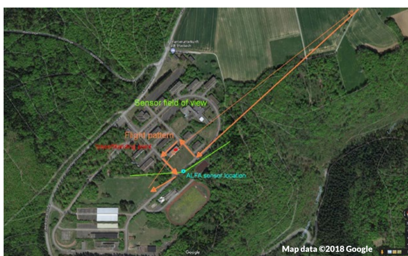
Drone flight pattern with position markers (red dots) of the drone pilots.
